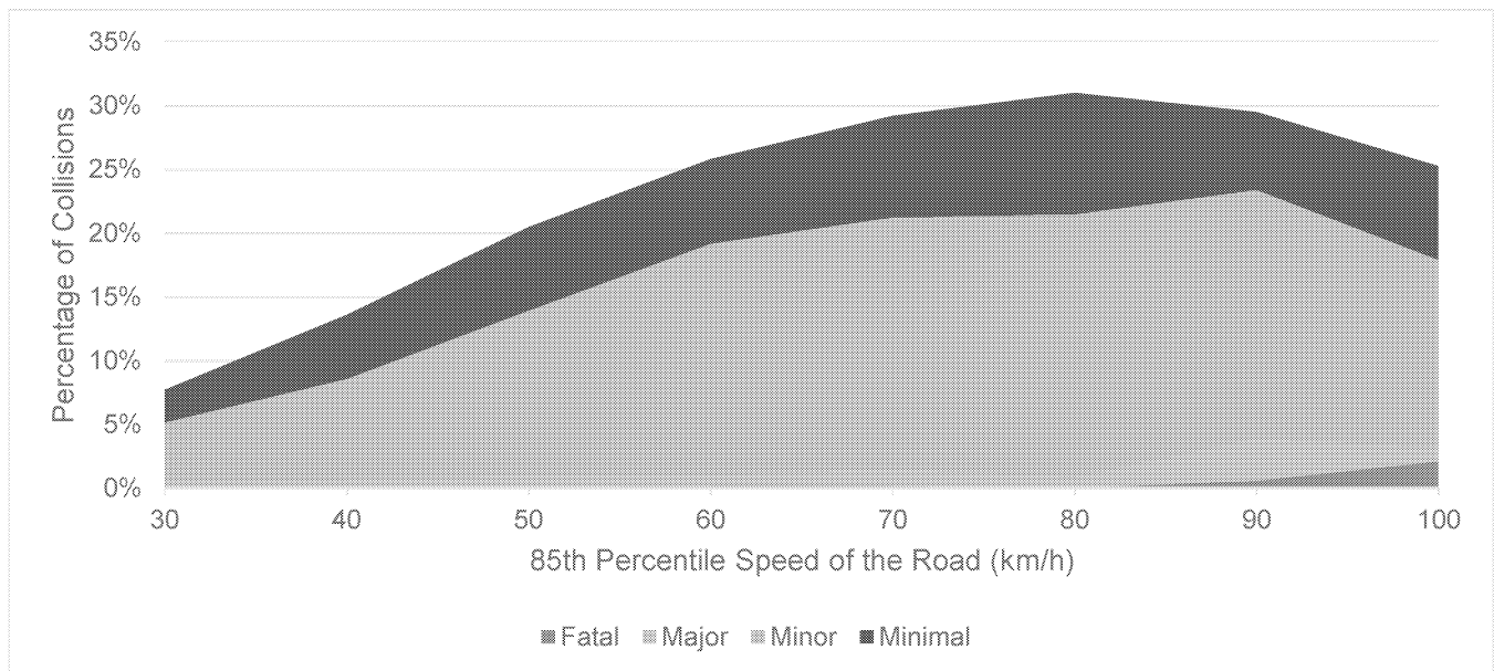
Figure 4-6 Relationship Between Turning Movement Collision Severity and Operating Speed
